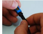
3: Fiber insertion & push the hold button to fix the fiber
